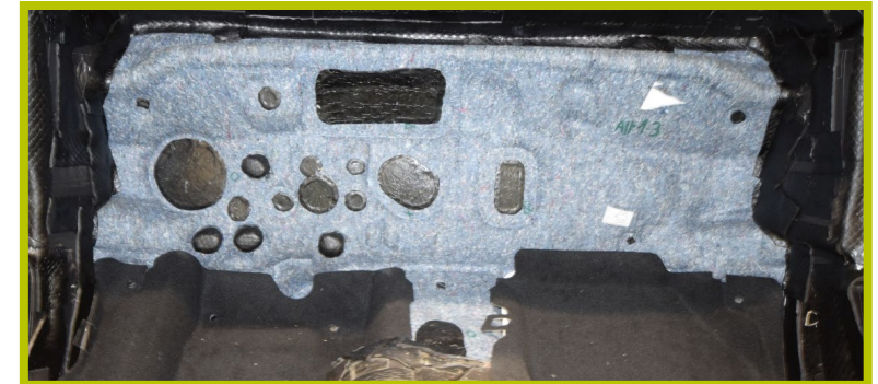
Heavy Layer + PU Foam HL 2.0kg/m2 + PUR 60kg/m3 + PET 400g/m2 noise-absorbing pad (total weight 4.95kg)
